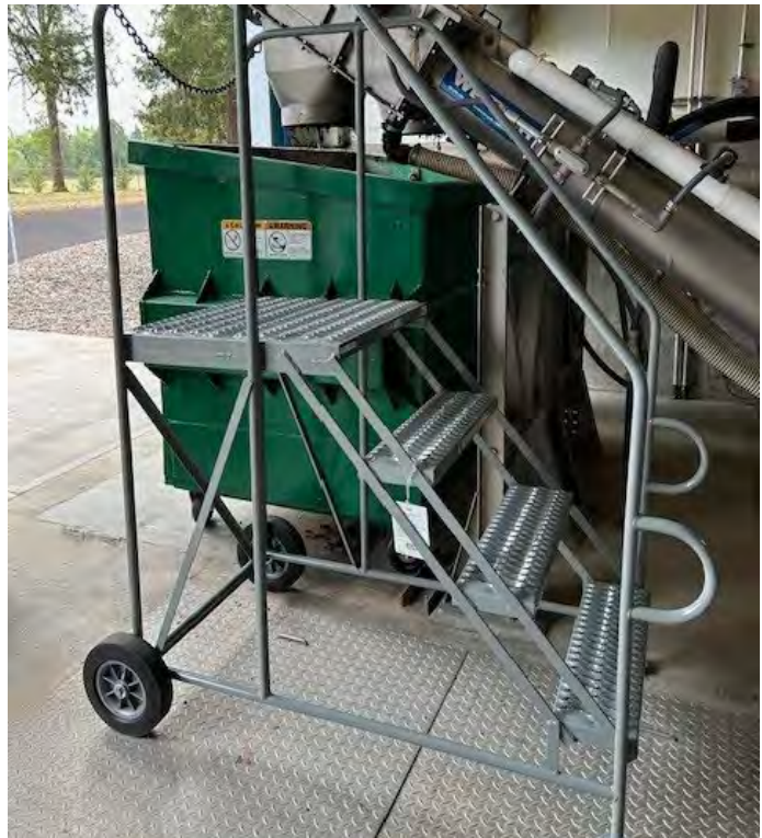
This ladder was replaced to improve stability while working in the headworks of the wastewater plant.
