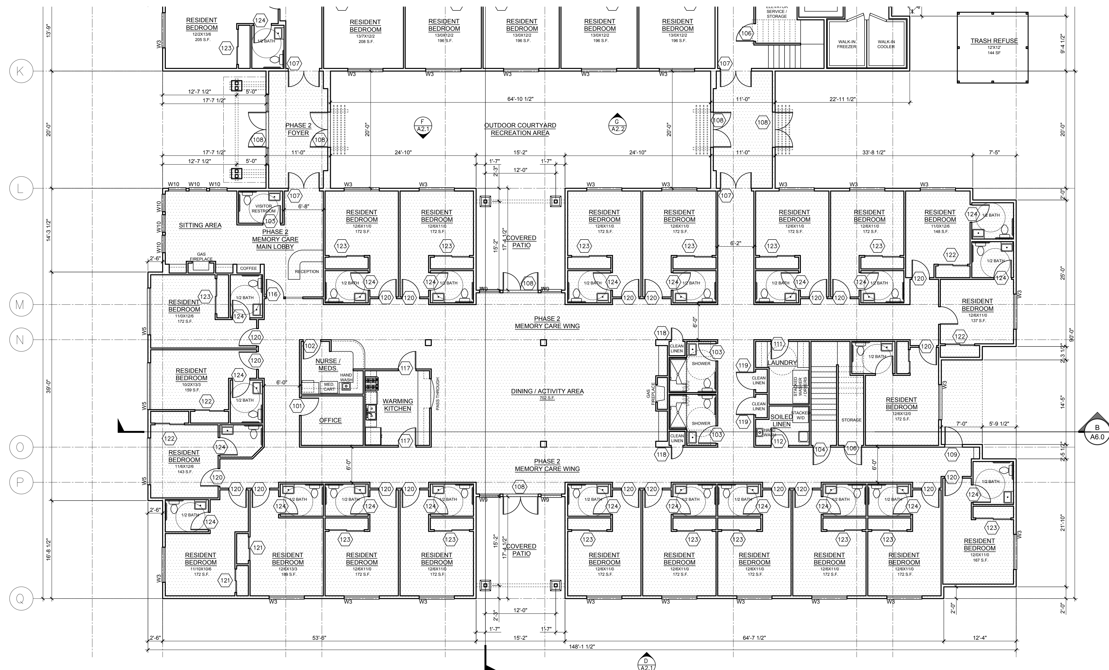
A A3.0 MAIN LEVEL FLOOR PLAN SCALE: 1/8" = 1'-0" PHASE 1: 35 RESIDENT BEDS; FLOOR AREA: 19,129 S.F. PHASE 2: 22 RESIDENT BEDS; FLOOR AREA: 10,056 S.F. TOTAL FLOOR AREA (PHASE 1 & 2): 29,185 S.F. TOTAL BUILDING AREA: 56,480 S.F.
