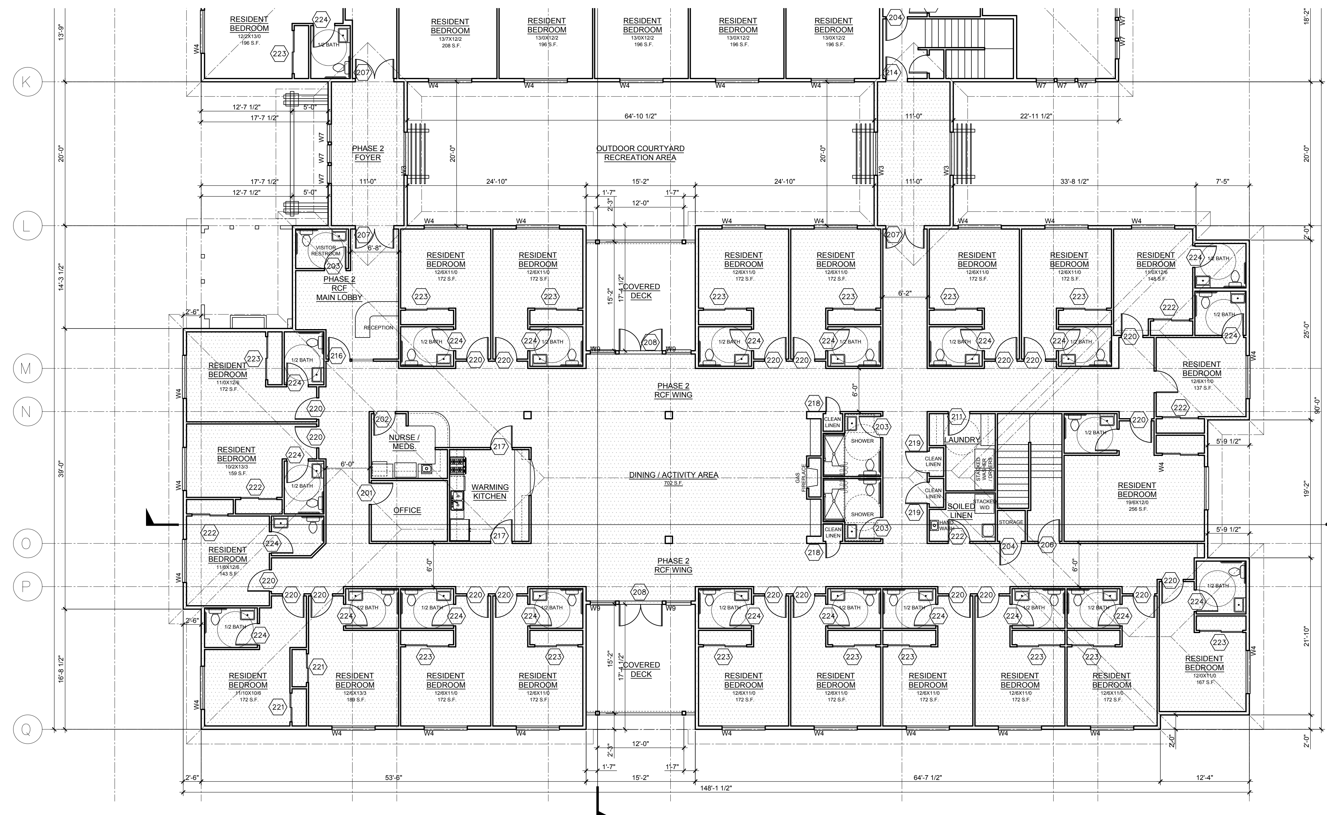
A A3.2 UPPER LEVEL FLOOR PLAN SCALE: 1/8" = 1'-0" PHASE 1: 35 RESIDENT BEDS; FLOOR AREA: 17,422 S.F. PHASE 2: 22 RESIDENT BEDS; FLOOR AREA: 9,873 S.F. TOTAL FLOOR AREA (PHASE 1 & 2): 27,295 S.F. TOTAL BUILDING AREA: 56,480 S.F.
