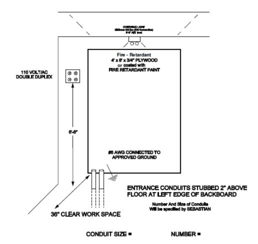
NOTE: Grounding source options are Electrical Power Service Grounding Electrode, Service Grounding Electrode Conductior or Service Panel, UFER, grounding ring, or driven ground rod.
